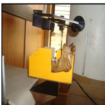
[Table/Fig-2]: The stainless steel wires attached to lines ab and cd [Table/Fig-3]: The photograph showing positioning of dry mandibles in panoramic machine [Table/Fig-4]: Traced image of panoramic radiograph and distances measured on dry mandibles
